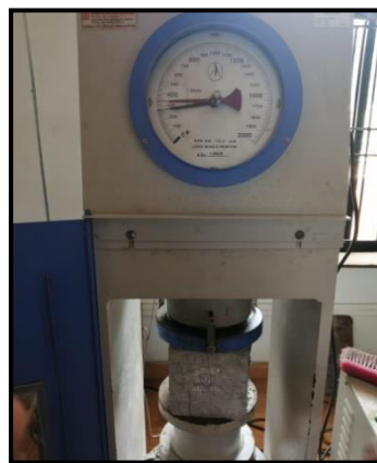
Fig 5: Compression test on cube specimen
