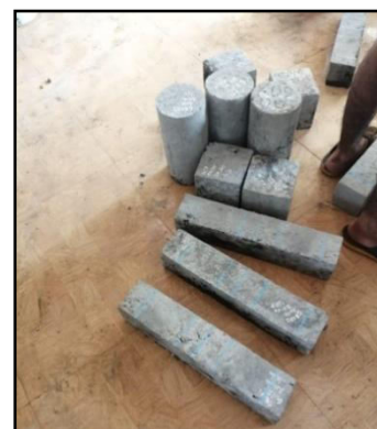
Fig 2: Specimens after 28 days of curing
