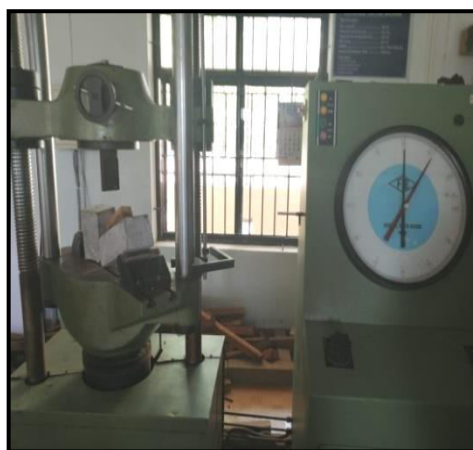
Fig 9: Flexural strength test on beam specimen
