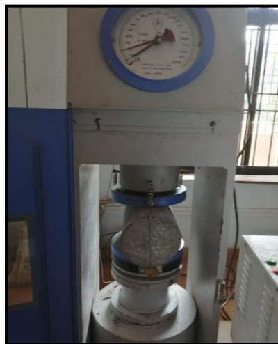
Fig 7: Split tensile test on cylindrical specimen
